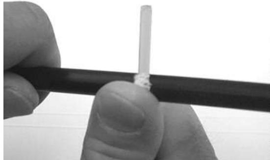
**Figure 2- Ring cut the cable jacket.**
